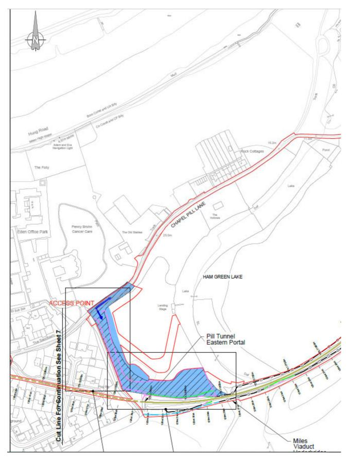
The plan as above also shows the access points proposed into the site during construction.
