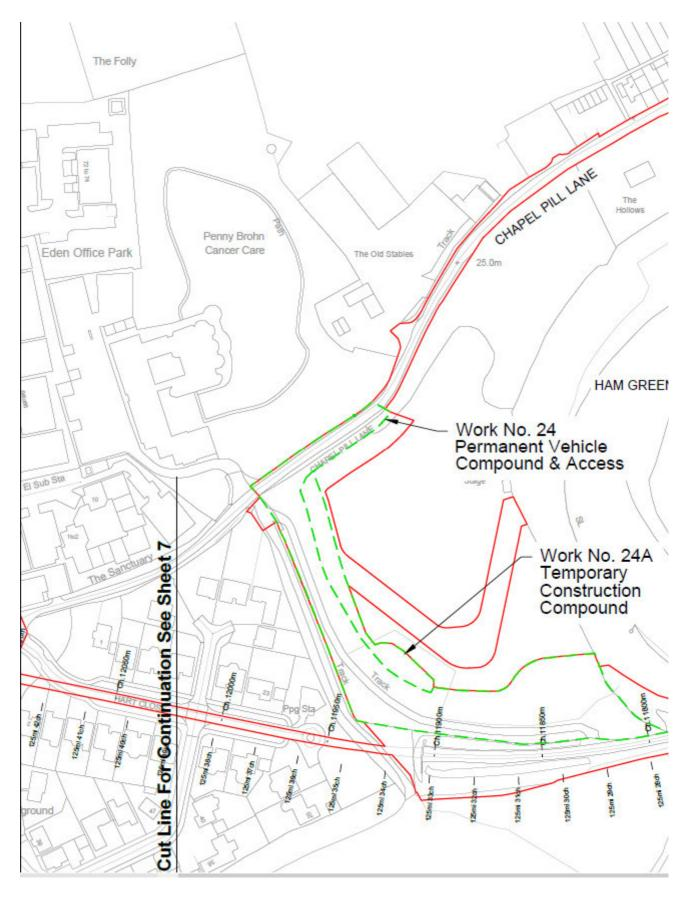
The green land shown on the plan as attached and as above is needed on a temporary basis to provide a work area to construct the permanent new access and compound and also to provide Mr Hunt with temporary access to his fishing lake during constrution of the permanent new access and compound areas shown in pink on the attached plan.
